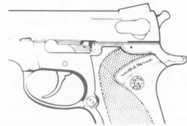
(Figure 4) Fire Position - Left Side Safety
